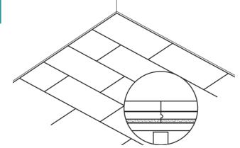
Continue to lay the Monarfloor® Tri-Board over the existing floor in a broken bond pattern, applying Monarfloor® Adhesive to all tongue and groove panel joints.
