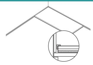
Starting from the furthest point out of each room, lay the first Monarfloor® Tri-Board over the sub-floor perpendicular to the floor joists, butting the edges tight to the Monarfloor® Flanking Band.
