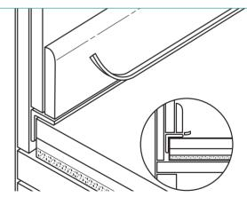
When the floor is fully covered install skirting and trim off excess Monarfloor® Flanking Band.
